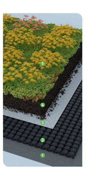
The basic principle of the green roof superstructure is always the same. However, differences may be necessary due to the type of building or the roof itself. This is why we offer various system solutions and therefore the right solution for every requirement.
